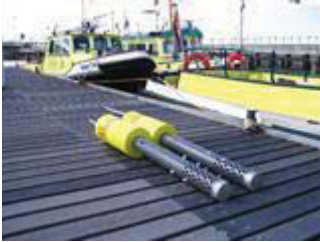
Data Buoy with Data Logger OMC-045-B-250
