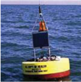
EMM700 Water Quality Monitoring Buoy
